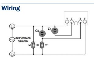
Model Name ECS224L Operating voltage AC 220V, 50/60Hz Application CSIR or CSCR Motors (0.18~3.7kW)
