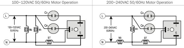
Model Name ECS112PS Operating voltage AC 110V, 50/60Hz Application RSIR Motors (0.18~1.1kW)
