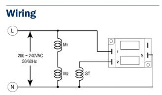
M1/M2: Main coil, ST: Auxiliary coil
