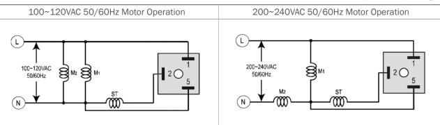
M1/M2: Main coil, ST: Auxiliary coil
